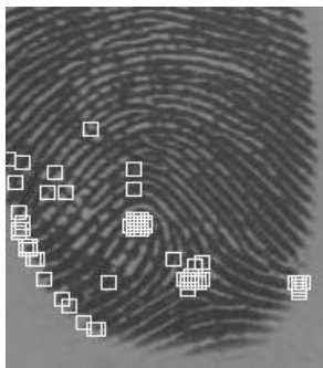
Fig.3 Singularities detected by block images through shifting position of the whole image time after time at the same block size (8 \times 8) 图 3 在同一分块尺寸 (8 \times 8) 下进行多次错位分块后检测的奇异点
