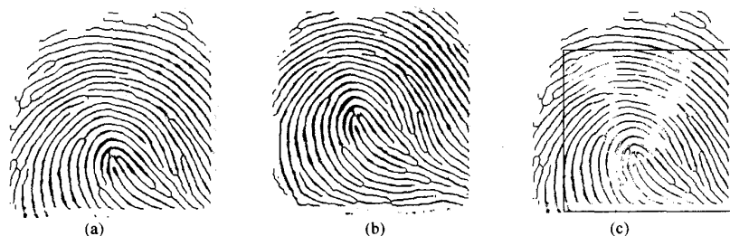
Fig. 5 Overlap of thinning fingerprint images after alignment. (a) Template image; (b) Input image; and (c) Input image aligned is mapped into template image, (c) overlap of the two fingerprints.
