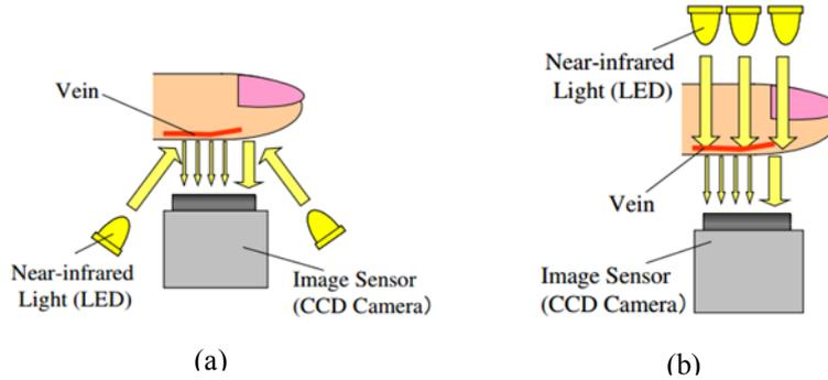
Fig.2 Two ways of finger vein image acquisition [2]:
